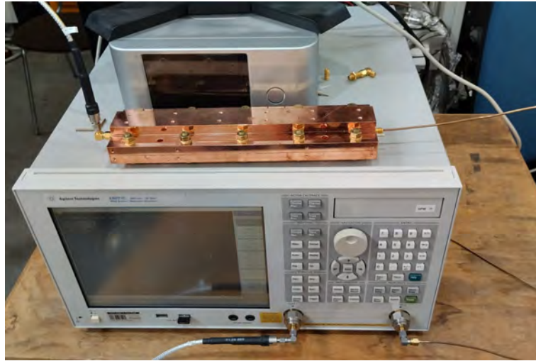
Figure 3.18. [53] Measurement apparatus that leads to the transmission coefficient shown in Fig. 3.17, the VNA provides the RF input and it allows us to directly measure the output signal coming from the resonant cavity.
