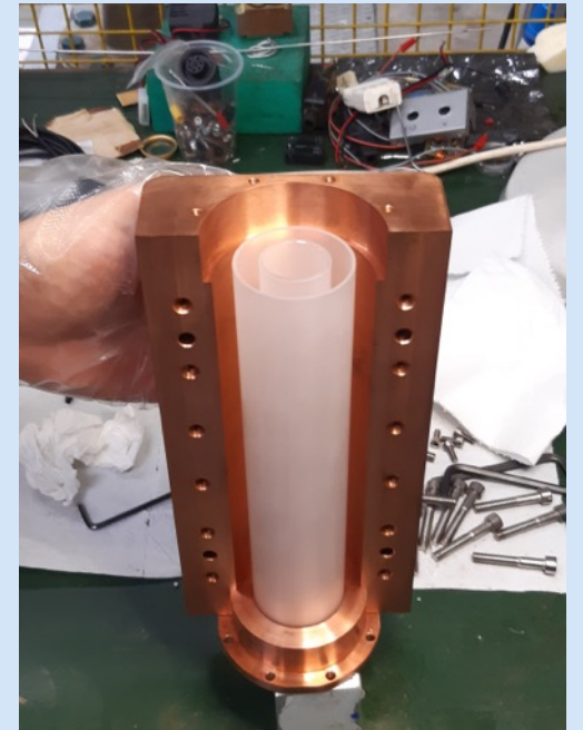
High quality factor photonic resonator with hollow dielectric cylinders
